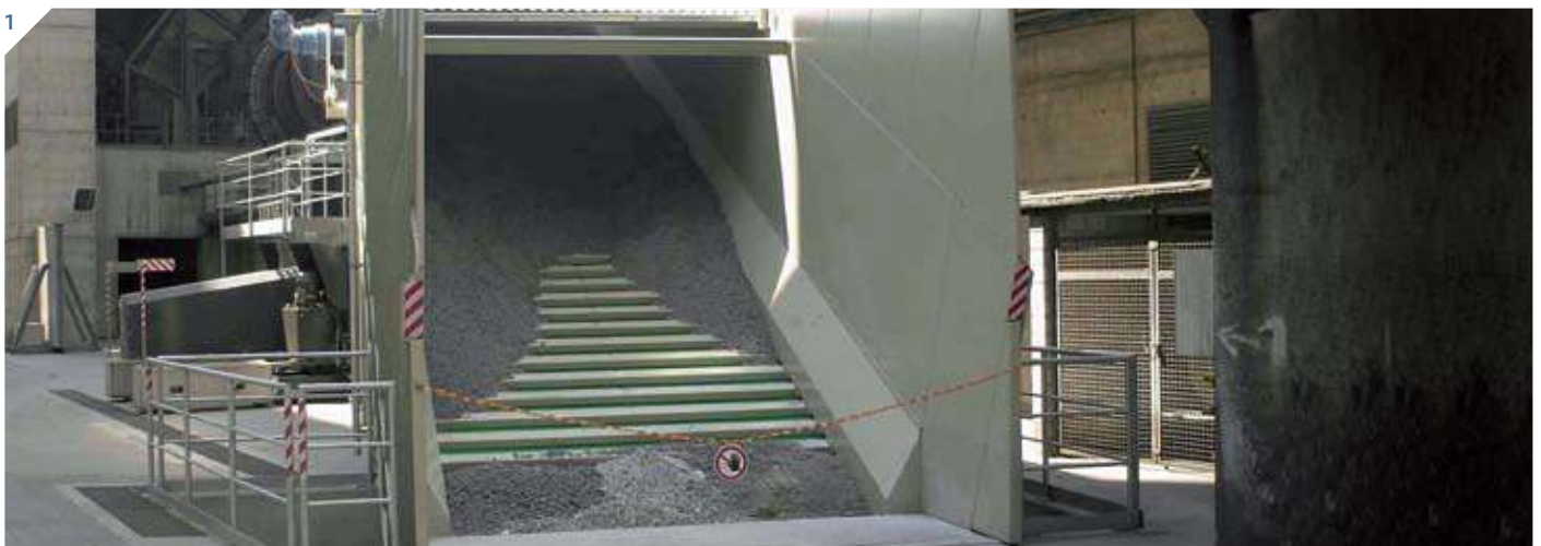
1. At Jura Cement's Wildeggen plant in Switzerland alternative fuels, including the paper sludge pictured, provide over 50% of the energy required for clinker production.
