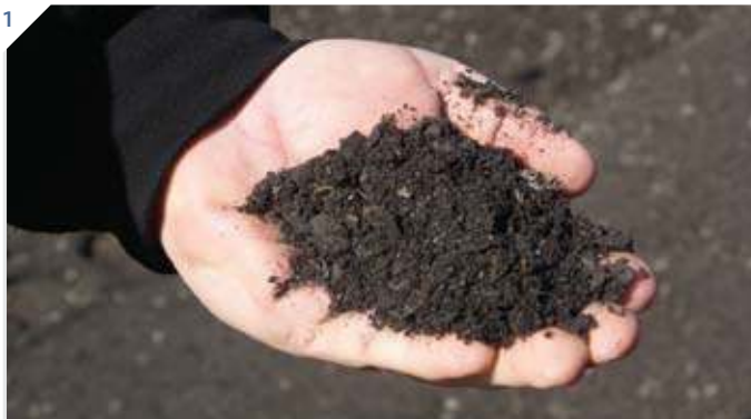
1. APAC-Texas Bitulithic, USA, utilises recycled asphalt-containing roofing material (shingles) in the production of asphalt.
