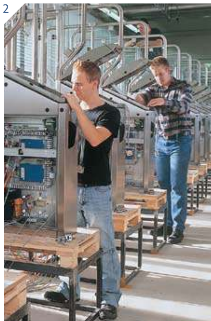
2. Products: Skilled specialists at Magnetic Autocontrol, Germany, assembling fare collection access control gates.
