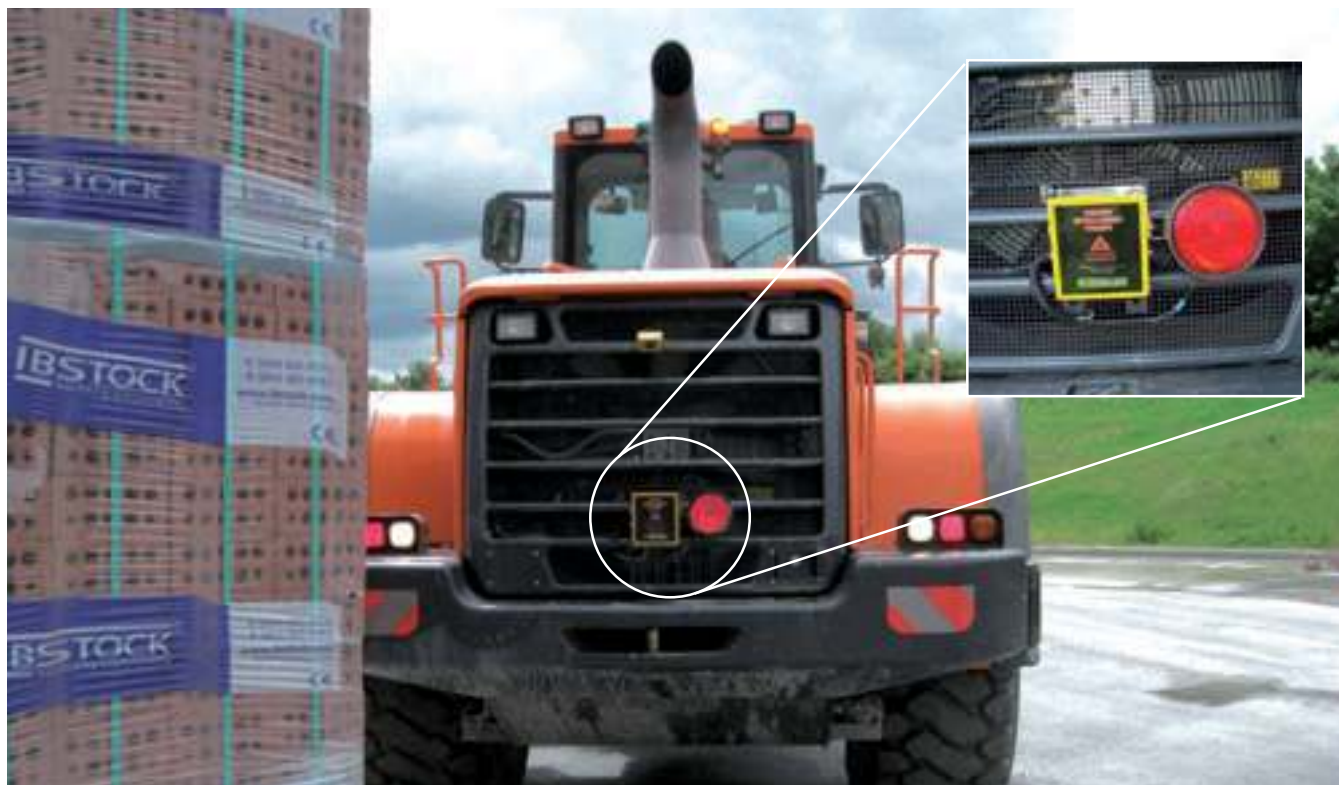
A rear facing radar detection system fitted to a loading shovel at Ibstock's clay brick plant at Throckley, UK.
