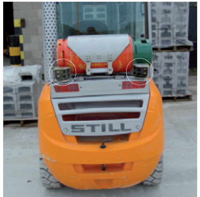
Ibstock and Forticrete, UK: prototype forklift with sensors interlocked with the braking system under test.
